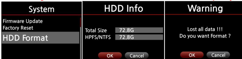
⑥ X10 re-boots automatically after finishing HDD format.
